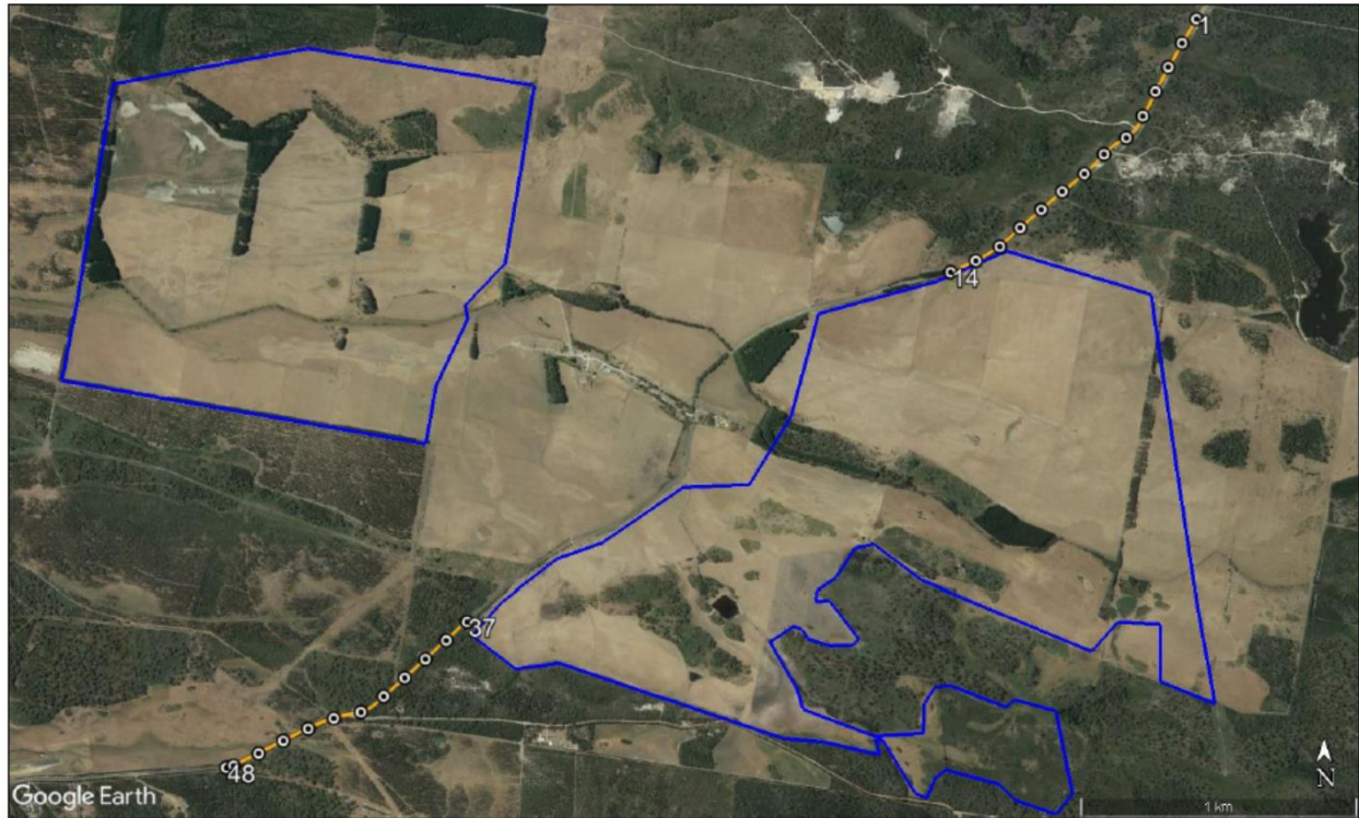
Figure 50. Sections of Soldiers Settlement road (shown in orange) from which solar reflections are geometrically possible.
